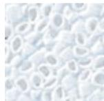
Sound absorptive panels are now available made from porous expanded polypropylene. The surface looks like many small cylindrical pellets bonded together. The advantages of the panels are their durability and washability. They can be used in many areas where other materials are not suitable for the environment. They are even somewhat rigid structurally and resistant to bacteria and fungi. The disadvantage is poor low-frequency absorption.
